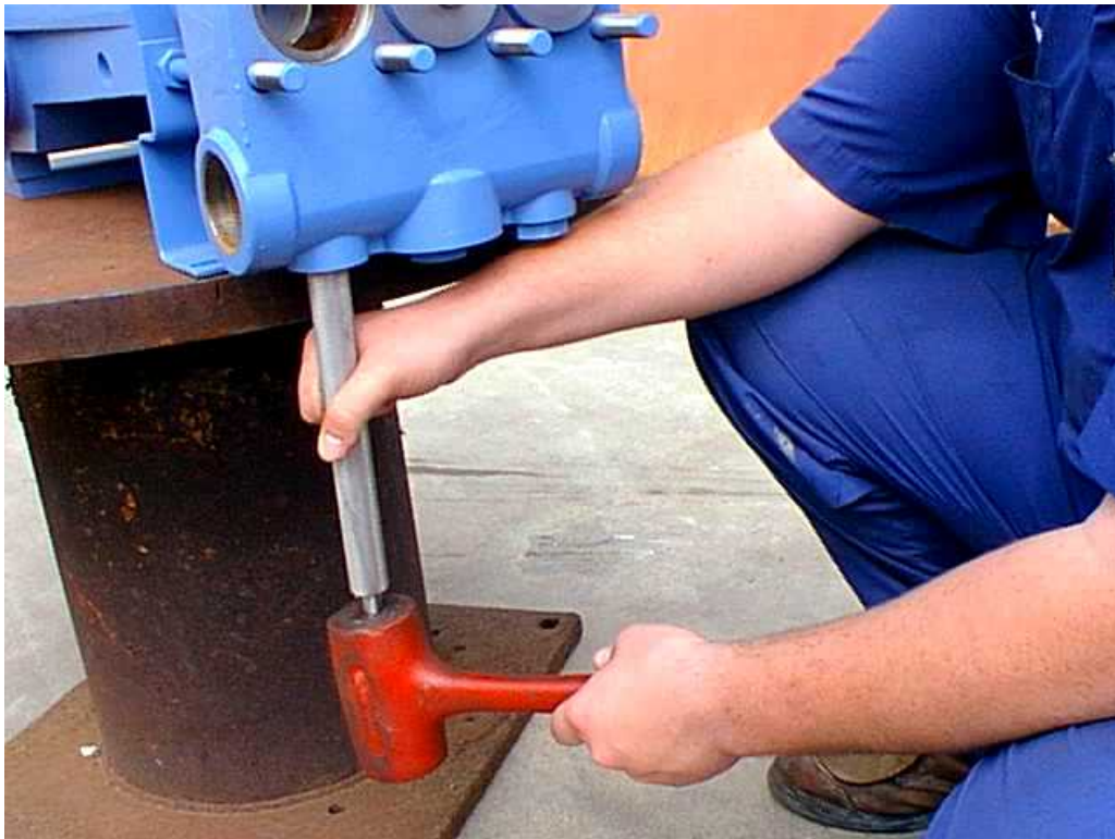
Picture 1: Removing the valve from the seat
